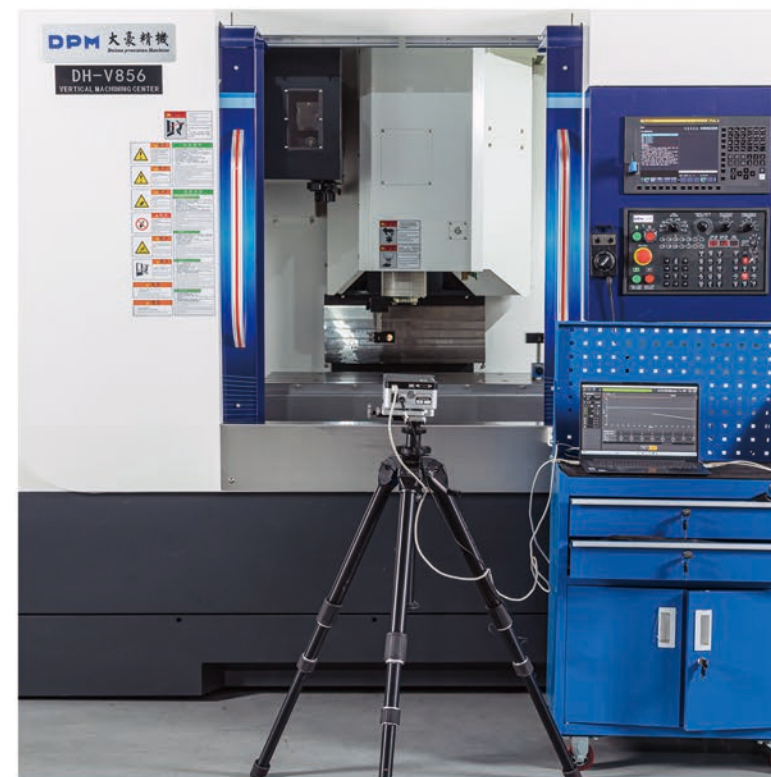
鐳射校正及循圓檢驗，動平衡校正 Laser calibration and circular inspection, dynamic balance calibration
